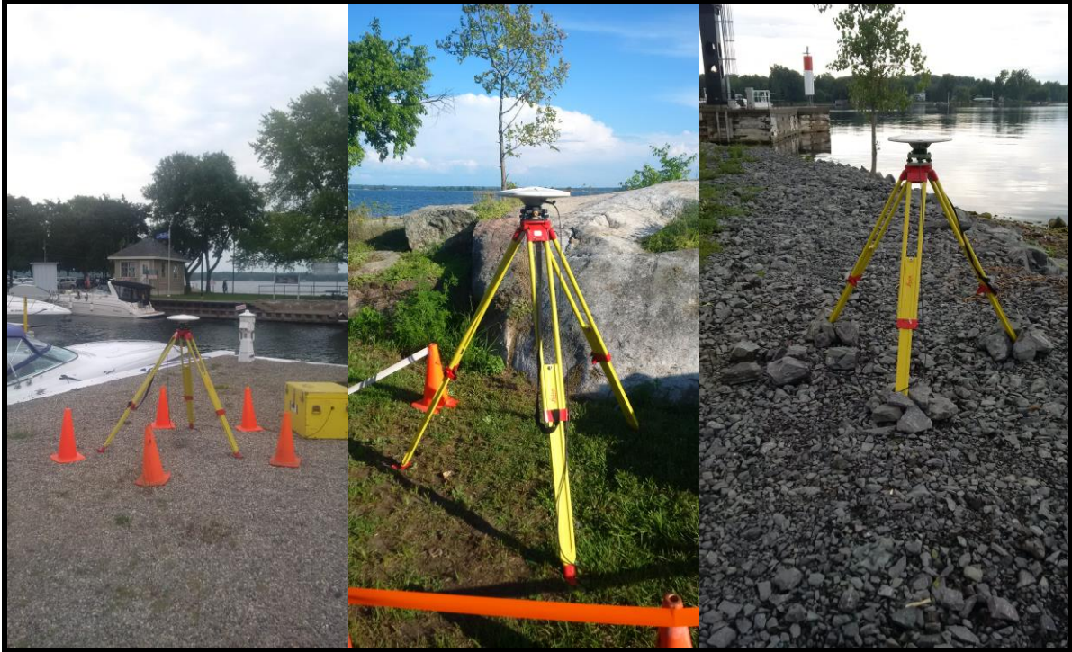
Figure 4 – Trimble R7, PPK GPS Reference Stations; Left to Right: Station TALL (Brockville), Station TINP (Mallorytown) and Station HIFD (Howe Island Ferry Dock)
