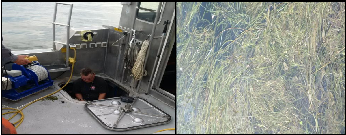
Figure 11 – Left; Logan cleaning out kelp/grass clogging the intake. An ongoing nuisance
